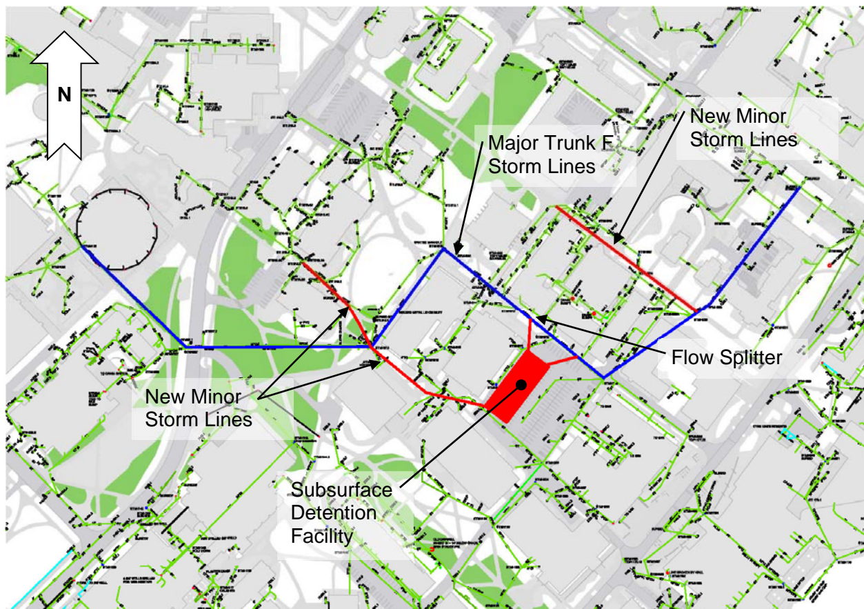
Figure 6.t. Recommended Improvements in the Trunk F Area
