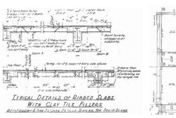
Typical Ribbed Slab with Clay Tile Filler Detail
